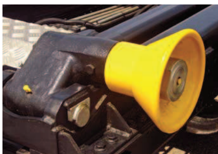
Cast steel rear roller for long lifetime
