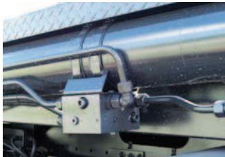
Check valves on each hydraulic cylinder
