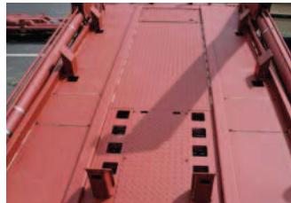
Adjustable container stops – lengthwise / sidewise
